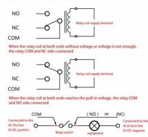
When the relay switch is closed, the device has a voltage at both ends, can work properly, switch off does not work
